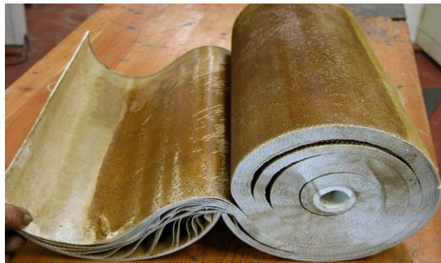
A cut up RO membrane showing uniform layers of manganese oxidizing bacteria
